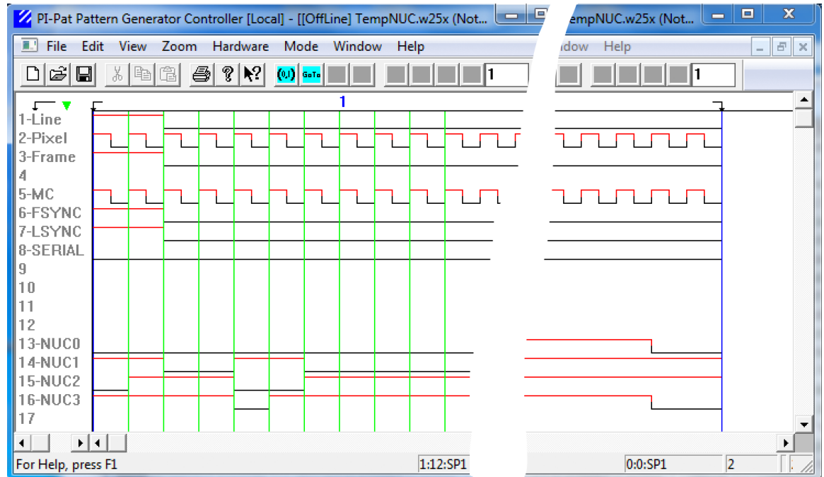
Figure 40: NUC Pattern Injection data in PI-PAT (NUC File), Offset = +2
