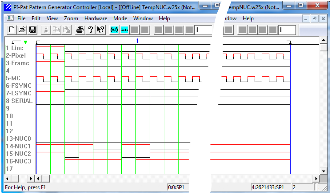
Figure 39: NUC Pattern Injection data in PI-PAT (NUC File), Offset = 0
