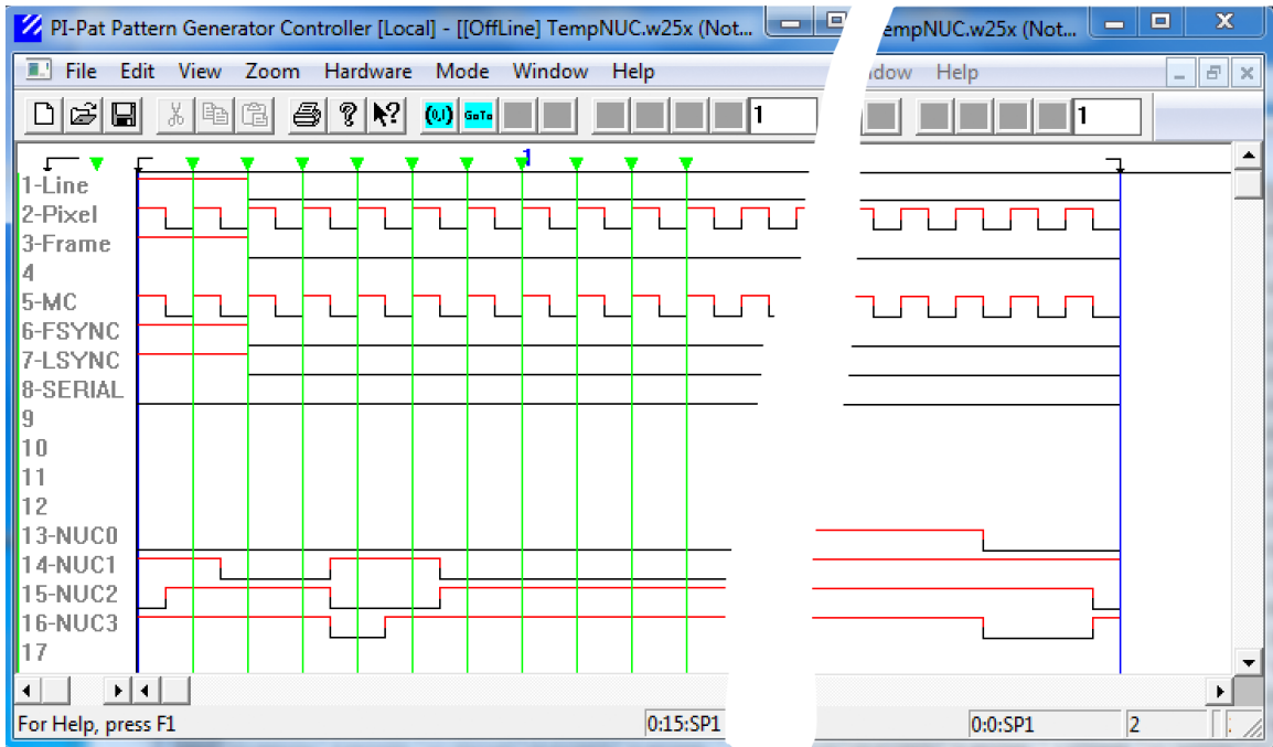
Figure 41: NUC Pattern Injection data in PI-PAT (NUC File), Offset = +2.5
