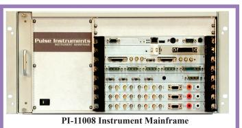
single-board-computer or bus extension card with the remaining 7 slots available for instrument cards from Pulse Instruments or other vendors.<sup>1</sup>
